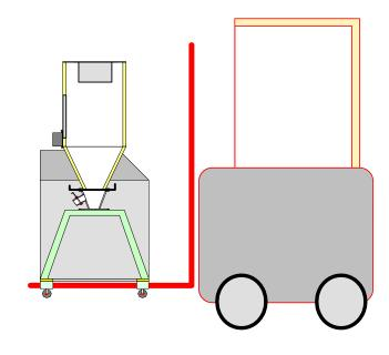
**Caution!** Do not use a hoist to move or rig your Drying/Conveying System when it is mounted on a cart! Moving the unit with a hoist will cause it to become unstable and may cause damage to the equipment and/or injury to personnel!
